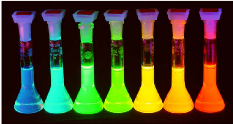
Figure 1: Illustrated the Colloidally prepared cedes quantum dots of different sizes [10].
